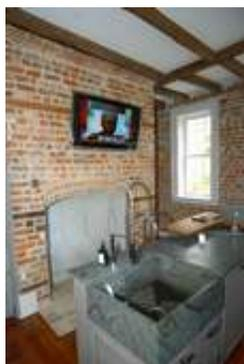
The kitchen was restored with modern features while keeping the old chimney. Wiring was installed behind the walls before the bricks went back up so a television could be installed.
